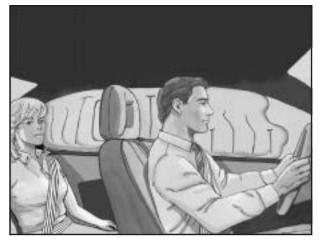
If your vehicle has a roof-mounted airbag for the driver and the person seated directly behind the driver, it is located in the ceiling above the side windows.
